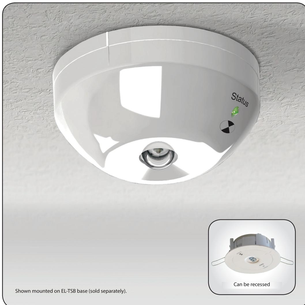
EL-DL3-AS is an LED-based, addressable open space down light featuring one high-powered LED with a specially engineered dual surface free-form optic. The unit's body contains the electronics and the stand-by battery and features a bicoloured status LED indicating charge/fault status (green for charging, red for fault).
